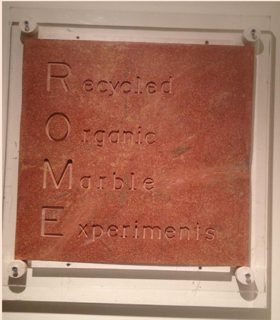
Photo 5 “Rosso antico” marble-like tile in wood pulp. The R.O.M.E. “logo” is the acronym for Recycled-Organic-Marble-Experiments
